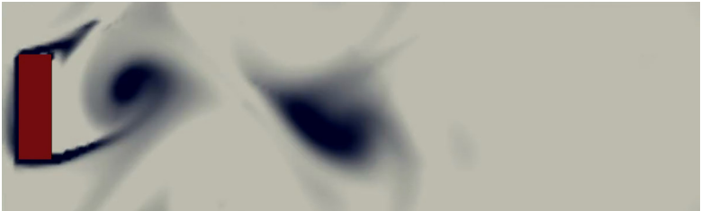
(G. Rempfer, C. Holm; ink droplet in a carrier fluid moving around a solid obstacle)
